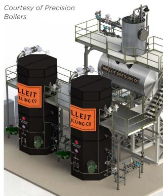
Modulation of the steam output is based on water circulation from the variable speed circulation pump. The boiler pressure control system modulates the pump speed and allows the boiler system to maintain constant steam pressure.
