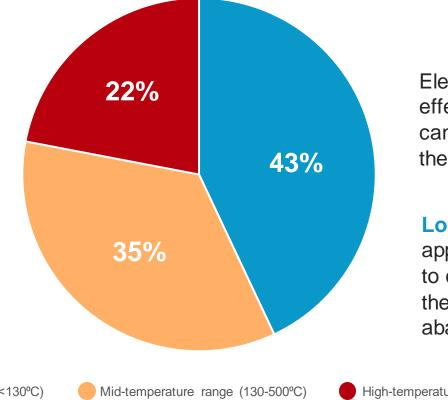
Electric heat pumps are effective under ~130°C and can target ~43% of industrial thermal energy use
